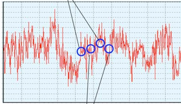
Fig. 9.4: Low-Frequency Noise Eliminated By Zero-Drift Amplifier
