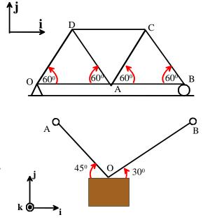
**4.5** The figure shows a heavy box suspended from two cables. The box is subjected to a vertical gravitational force, and two forces of magnitude  $T_1$ ,  $T_2$  acting parallel to cables OA, and OB, respectively. Express each force as vector components in the basis shown. Write down the vector sum of the forces.
