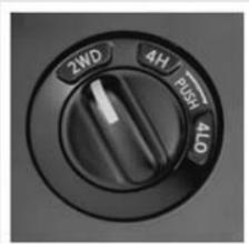
NOTE: The vehicle must be stopped and in N (NEUTRAL) with the brake pedal depressed when shifting into and out of 4LO.
