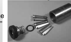
Strand Chuck Showing Internal Components
