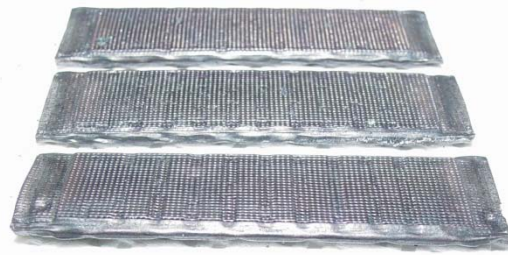
Steel pockets holding active material powder
