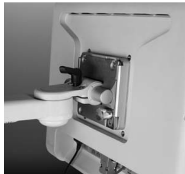
Figure 10 – Adjusting the touch screen tilt
