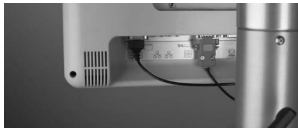
Figure 7 – Connecting the touch screen cables Note: Actual connector style may differ from illustration
