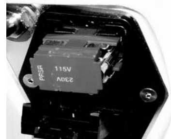
Figure 19 – Replacement Fuse Orientation: Orientation for 115V shown
