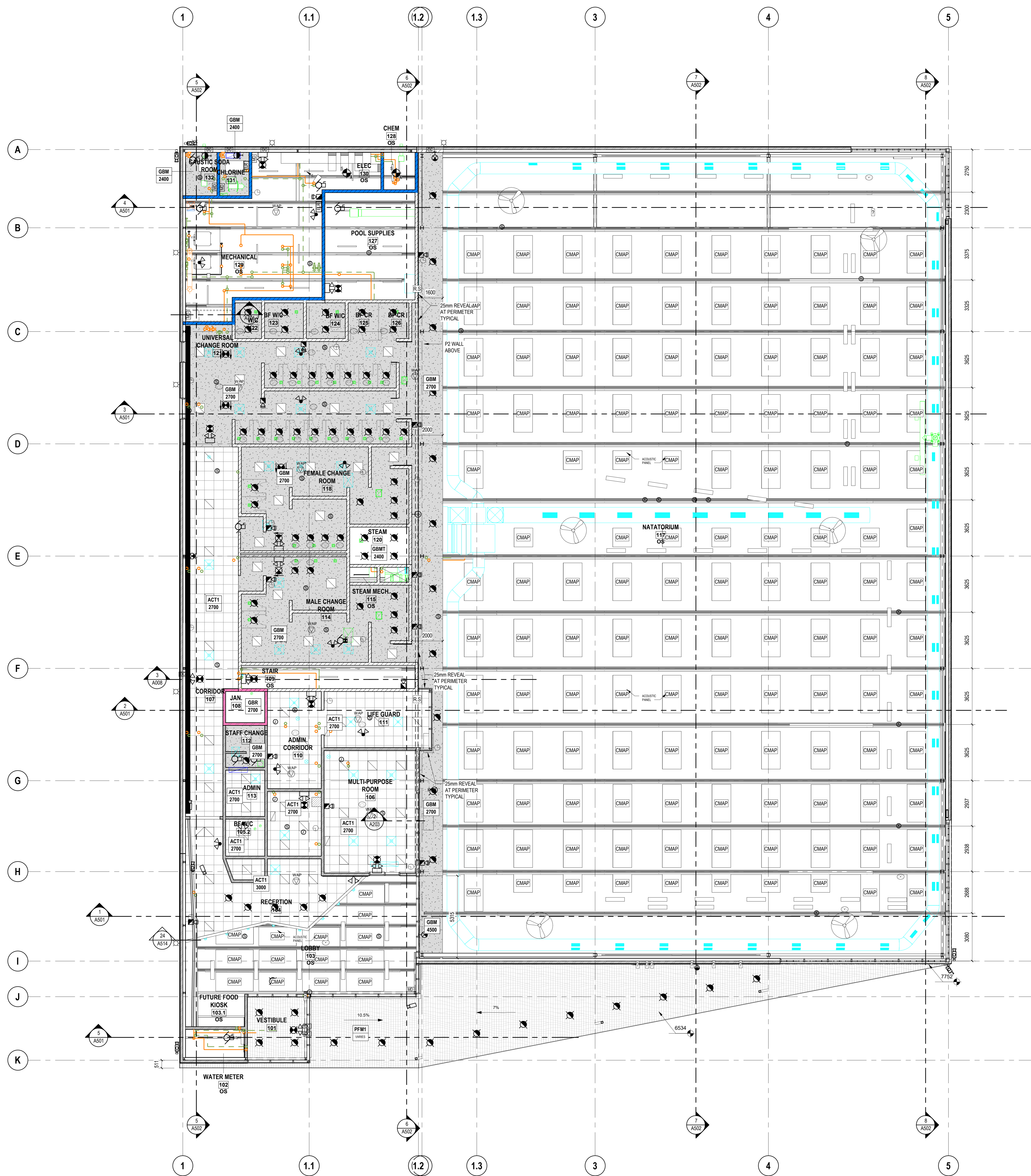
1 | MAIN FLOOR REFLECTED CEILING PLAN SCALE: 1:100
