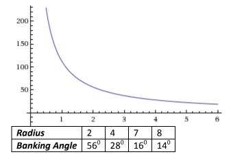
Which equation best represents the banking angle B for the turning radius r?
