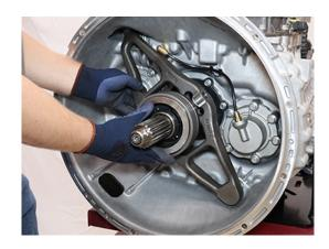
**2.** Pull to free the lower Clutch Release Yoke socket from the lower pivot on the clutch housing.
