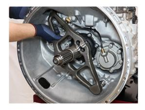
2. Install the lower Release Yoke socket over the lower pivot on the clutch housing and press until attached.
