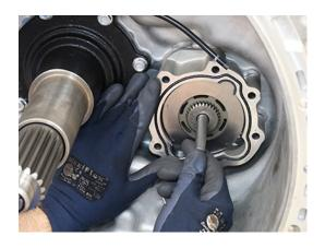
**5.** Install the Inertia Brake Cover onto the housing.
