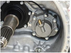
2. Remove the 6 Inertia Brake Cover 13 mm cap screws.
