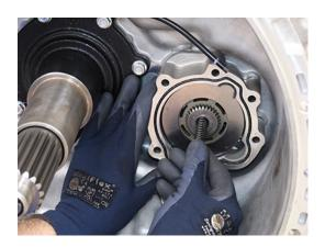
**4.** If removed, install the Piston Pin into the Lower Countershaft.
