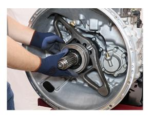
**4.** Push the upper end of the Release Yoke back until it locks to reset the LCA.
