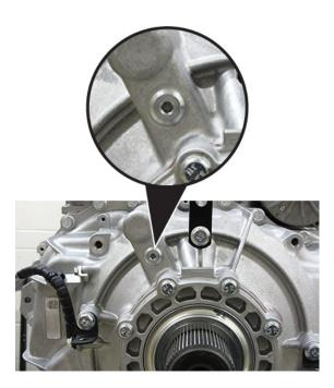
2. Place a suitable container under the Oil Check Plug and remove the Oil Check Plug with a 6 mm hex key.
