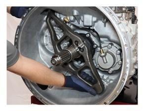
**3.** Pull to free the upper Clutch Release Yoke socket from the Linear Clutch Actuator (LCA) rod end.
