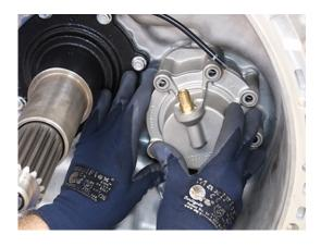
2. While holding the Inertia Brake Housing to the clutch housing, remove the Inertia Brake Cover.
