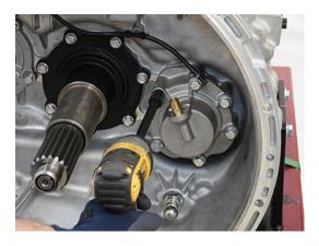
**3.** Remove the Inertia Brake Cover and Housing as an assembly. The original housing is not to be reused.
