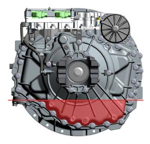
**4.** Inspect Oil Check Plug and O-ring for damage. If damaged, replace the Oil Check Plug; O-ring is serviced with plug.
