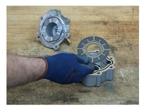
**6.** Place Inertia Brake Cover and Piston on the Housing. Align the bolt holes.
