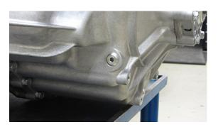
**3.** Fill the transmission with PS-386 lube until a small amount of oil runs out of the Oil Check Plug hole.
