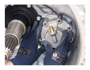
**4.** Ensure the Inertia Brake Piston Pin and Return Spring remain in the Lower Countershaft.
