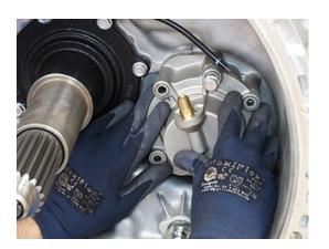
**6.** Install the six 13 mm cap screws and torque to 21-25 Nm (16-19 lb-ft) in a criss-cross pattern.
