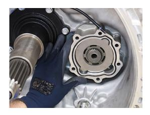
**3.** If removed, install the Return Spring into the Lower Countershaft.
