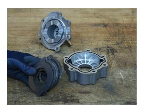
**2.** Remove the 2 wear guides from the Inertia Brake Housing.
