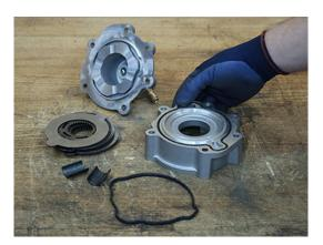
**3.** Insert the O-ring into the groove on the front of the Inertia Brake Housing until fully seated.
