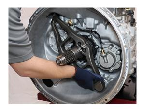
**3.** Slide the Release Bearing over the input shaft and into the Release Yoke.
