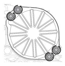
**4.** Tighten the 4 LCA to MTM T45 cap screws and torque to 23-27 Nm (17-21 lb-ft).
