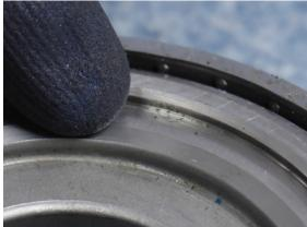
2. Insert the O-ring into the groove on the rear of the Inertia Brake Housing until fully seated.
