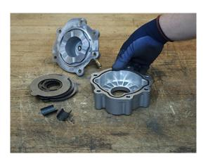
**4.** Install the 2 Wear Guides in the Inertia Brake Housing.
