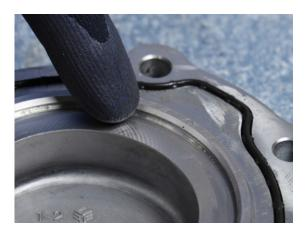
2. Install the new Upper Countershaft Cover O-ring (10001048) into the groove until fully seated.
