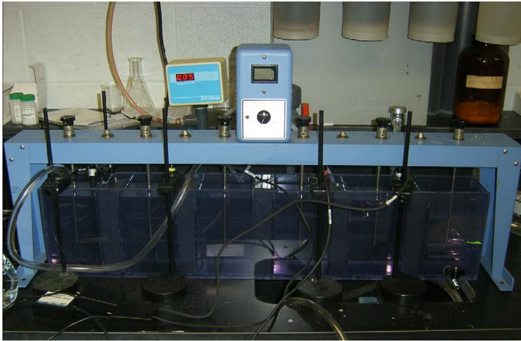
Figure 4: the 6 CSTRs in series reactor with stirrers and conductivity probes inside the series. Those probes have respectively been placed in the first, the second, the fourth and the fifth reactor
