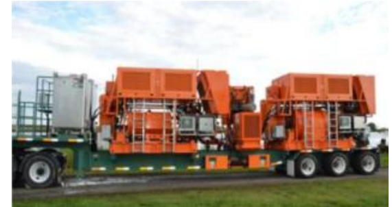
Latest generation turbine-powered pressure pumping unit (4,500 HP)
