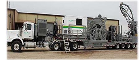
Coiled Tubing Unit
