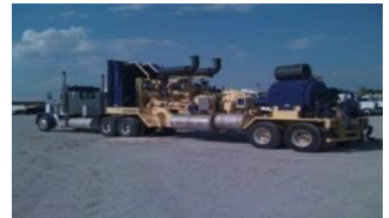
Conventional diesel-powered pump (1,800-2,500 HP)
