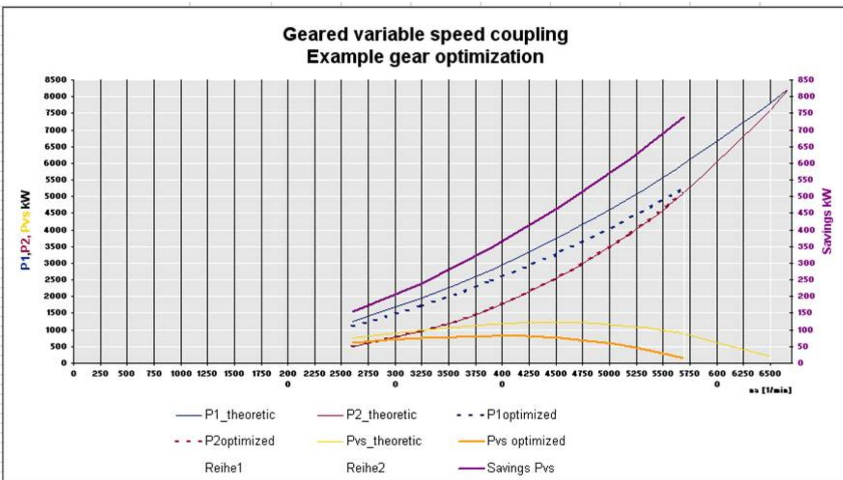
This diagram summarizes the layout data and the new operating point and shows the Pvs curves. The difference of these curves are shown as the power savings over the speed range. Taking into consideration that boiler feed pumps are operating approx. 8000 hours / year the investment will pay back after a short operating time.
