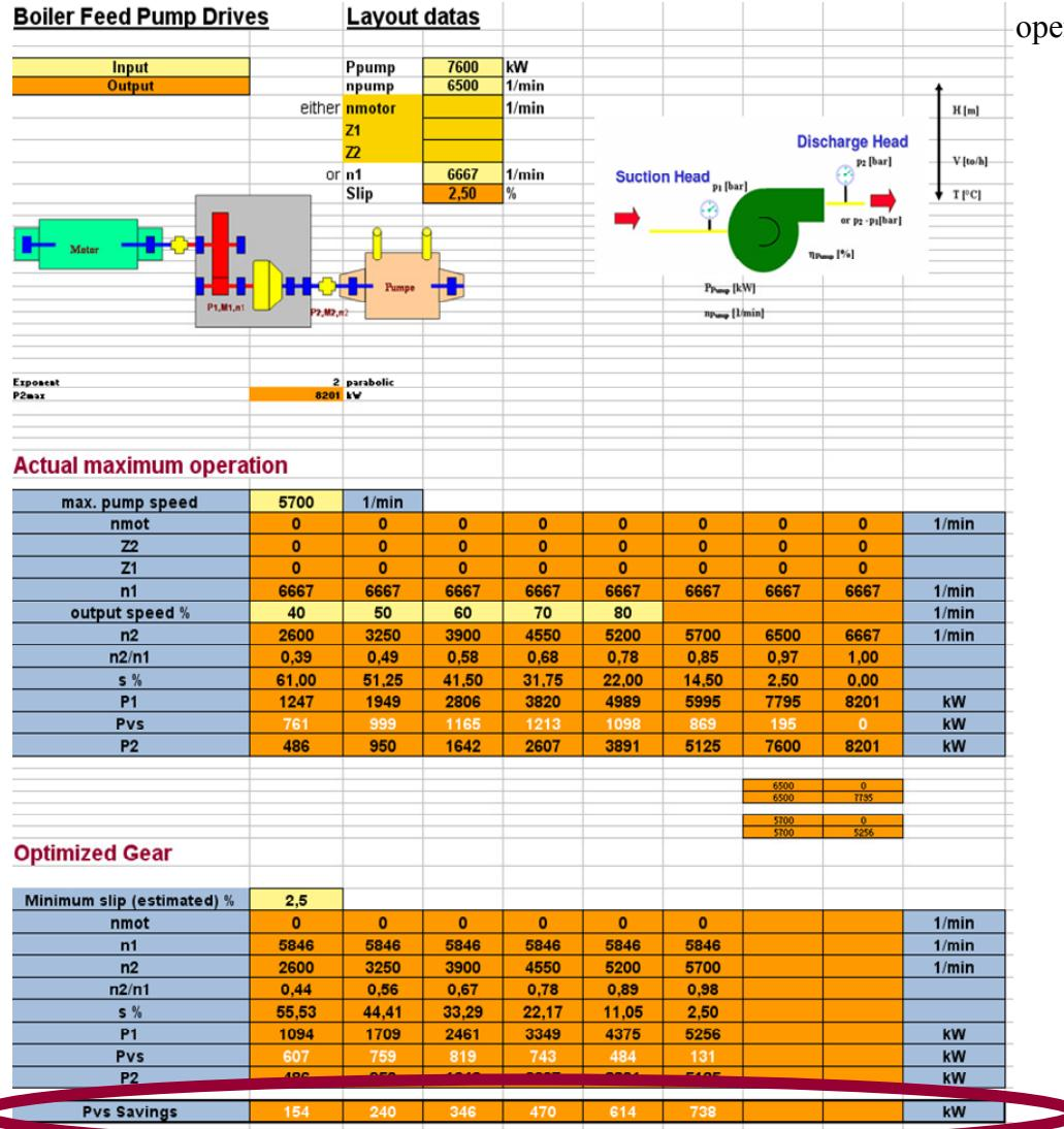
The improved condition with the optimized gear shows the possible power savings in KW per hour for a range of output speeds. This results in lower motor power consumption and represents the final operating savings.
