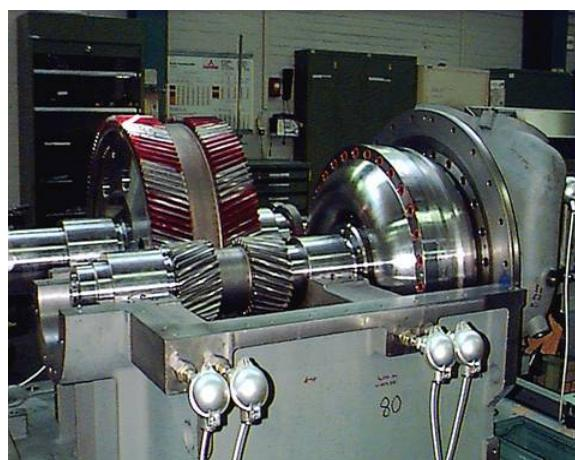
pumps is much lesser than the maximum possible speed. In this case the change of the step-up gear will result in reduced energy consumption. An easy pre-estimation for potential energy saving by a gear optimization can be carried out with a calculation program on site. Data which must be known are the original layout of the pump, the coupling type and size and the maximum pump speed ever needed.
