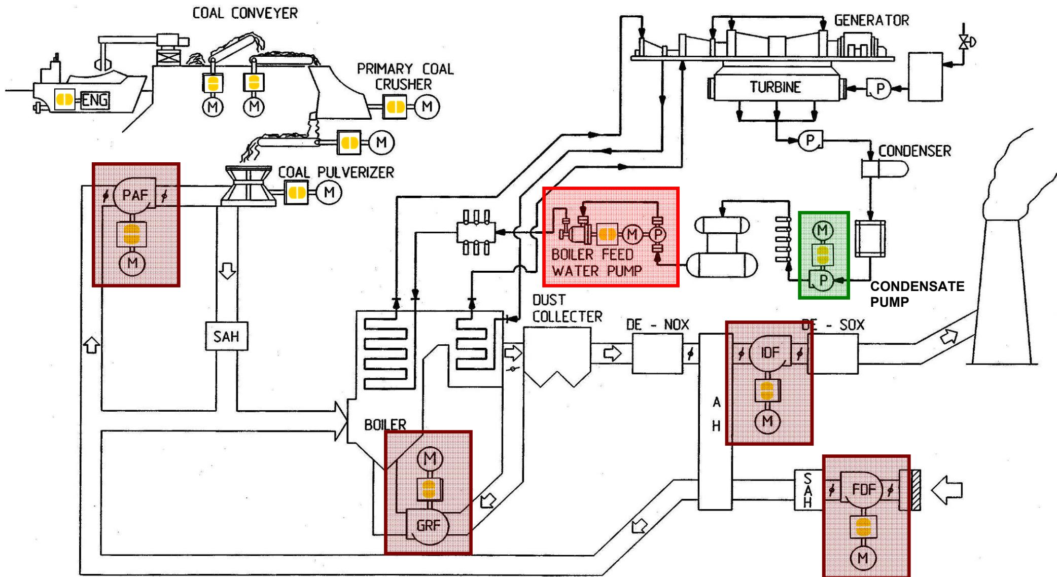
Attachment 2: Fluid Couplings in a Combined Cycle Power Plant
