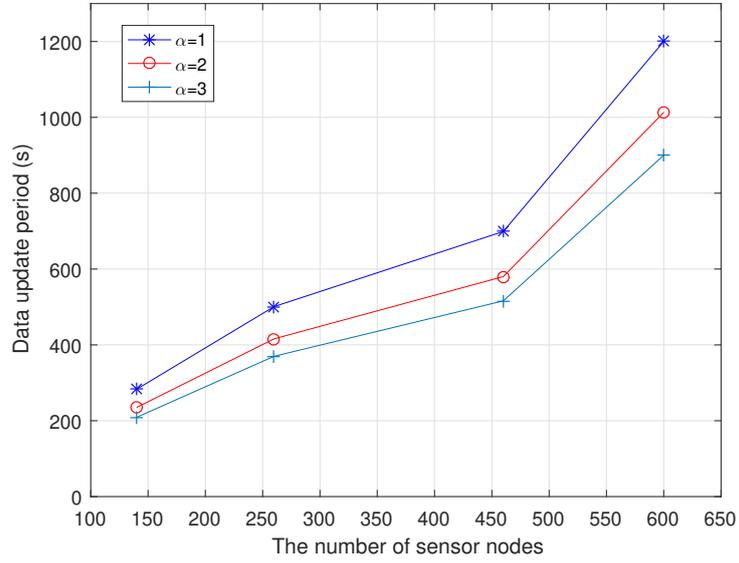
Figure 4.3: Comparison of data update period under different values of  $\alpha$
