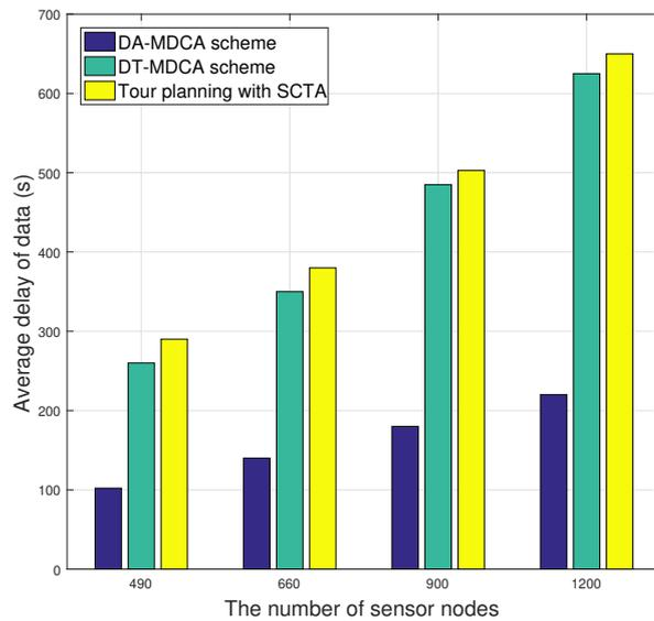
Figure 5.4: Comparison of the average delay of MDCA data collection schemes and the control group
