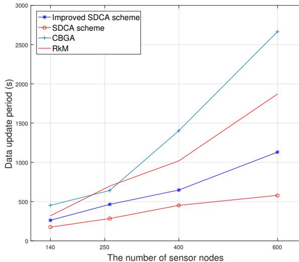
Figure 4.5: Comparison of data update period of the improved SDCA data collection scheme and the control group
