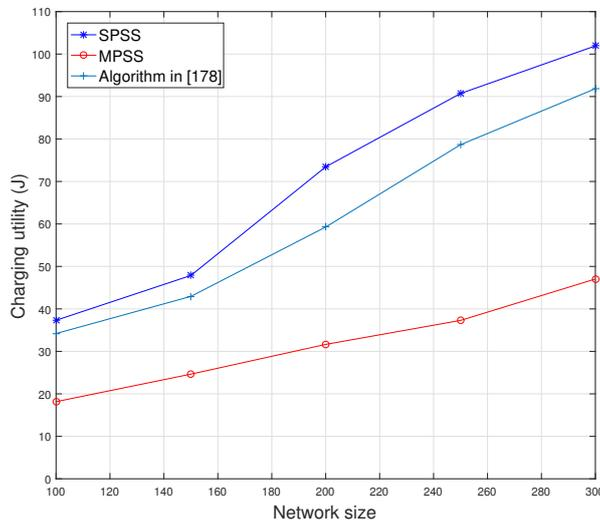
Figure 6.6: Comparison of the charging utility of joint data gathering and wireless charging schemes
