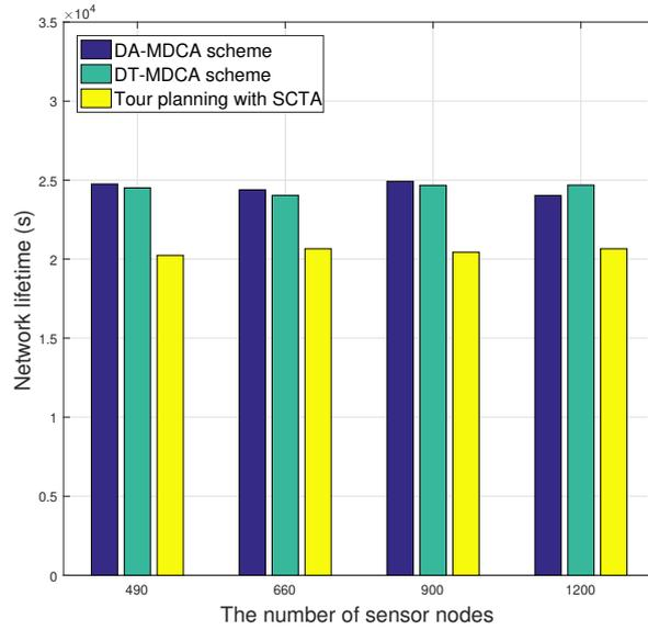
Figure 5.2: Comparison of network lifetime of MDCA data collection schemes and the control group
