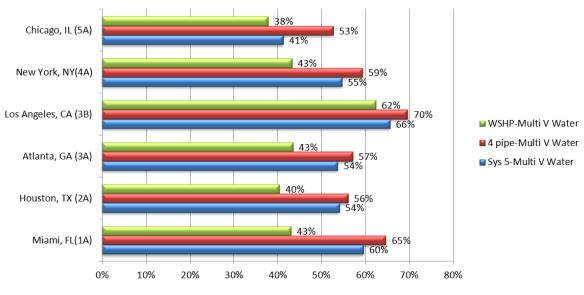
Figure 2 : LG Multi V Water IV VRF systems Whole Building Energy Cost (%) Savings.
