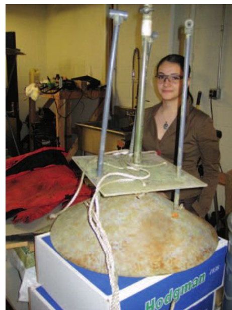
Alexandra Patricia Tcaciuc '08 displays an underwater gas-collection trap she helped design and build during her 2007 Martin Family UROP with Martin Fellow Charuleka Varadharajan (Civil and Environmental Engineering). Using these devices, they measured bubbling methane fluxes in Upper Mystic Lake in Woburn, Massachusetts, as part of a larger effort to quantify this source of greenhouse gas emissions. Tcaciuc is now a Martin Fellow herself.
