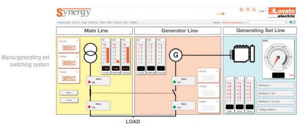
Single line layout of an electrical system
