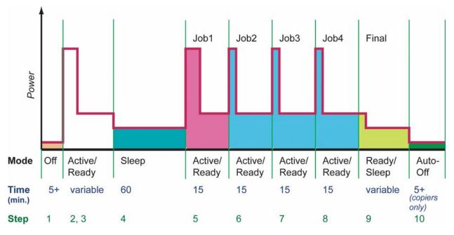
Figure 1. TEC Measurement Procedure
