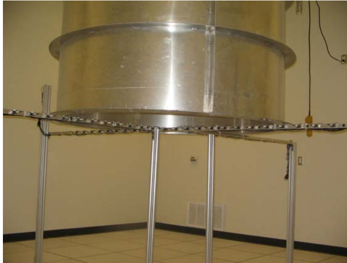
Figure 3.7 – Testing Cylinder, Sensors, and Sensor Arms (if using four fixed arms instead of single rotating arm)
