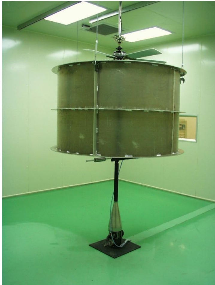
Figure 3.9 – Testing Cylinder and Chamber (if using single rotating arm instead of four fixed arms)
