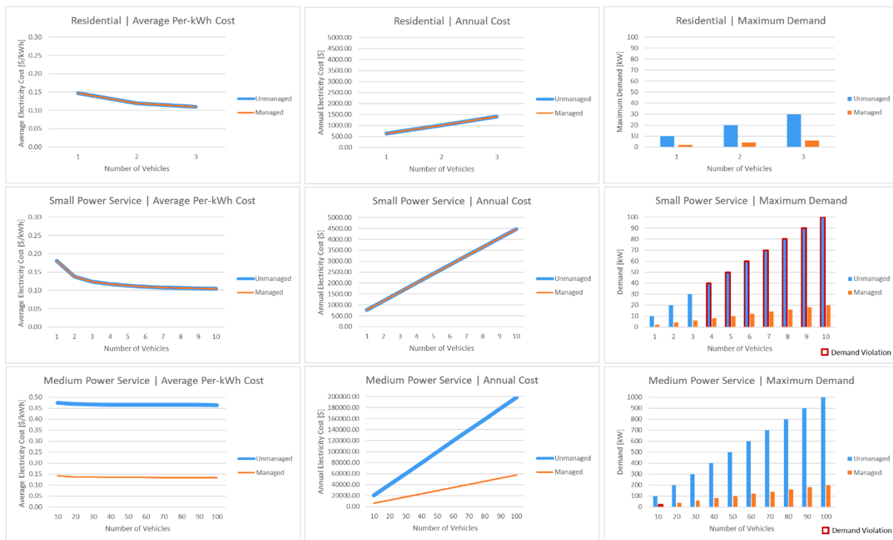
Panel of figures detailing average per-kWh costs, annual costs, and maximum demand for FAYPWC’s residential, small power service, and medium power service rates. Evening charging from 7pm to 6am is assumed for all scenarios (NCCETC 2020)
