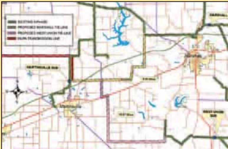
*Upon completion of the substation, EnerStar anticipates constructing two tie-lines, represented by a pink and a yellow line. When complete, the coop will link all EnerStar substations and have the ability to "back feed" subs during an extended outage.*
