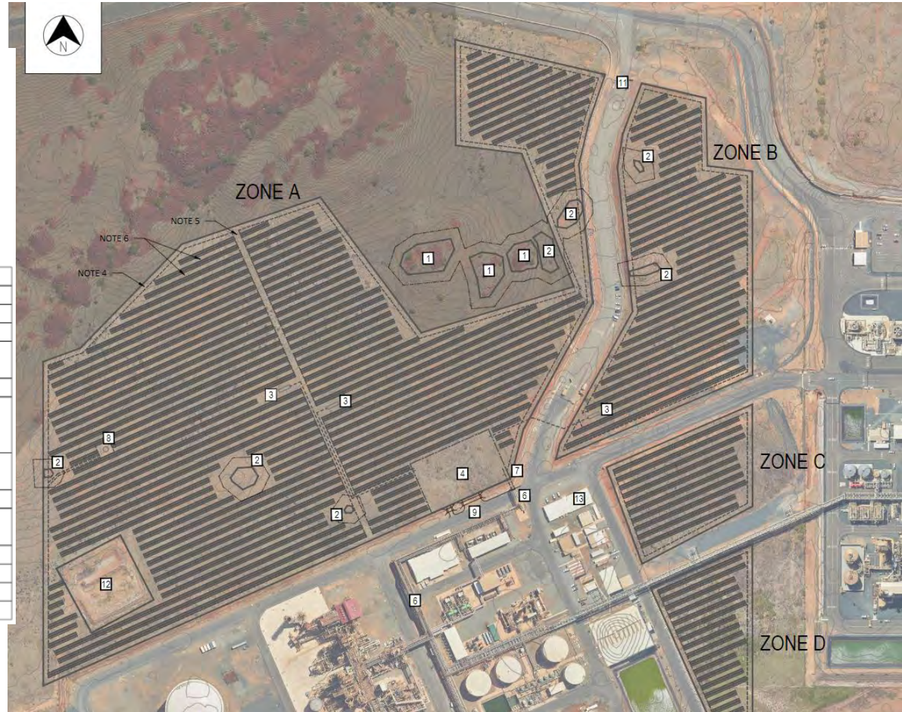
Figure 4: Solar Plant Layout (Jacobs)
