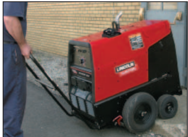
All-terrain undercarriage easily maneuvers over obstacles.
