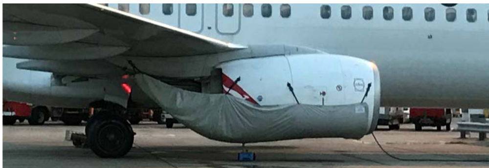
A new compressor wash system with detergent recovery.
