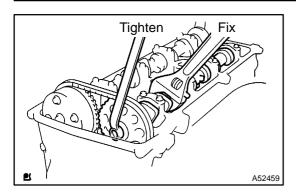
(4) Fix the camshaft with a wrench, then tighten the sprocket bolt.
