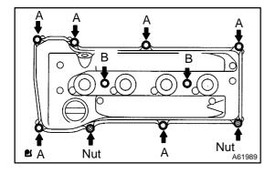
(c) Install the cylinder head cover with the 8 bolts and 2 nuts. **Torque:**
