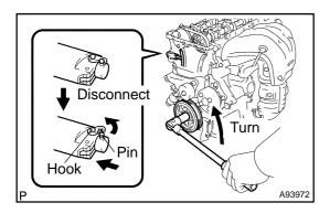
(3) Turn the crankshaft counterclockwise, and disconnect the plunger knock pin from the hook.
