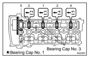
(2) Examine the front marks and numbers of the 5 bearing caps and install them. Then install the 10 bearing cap bolts. Uniformly tighten the bolts in the sequence shown in the illustration.
