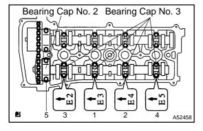
(3) Examine the front marks and numbers of the 5 bearing caps and install them. Then install the 10 bearing cap bolts. Uniformly tighten the bolts in the sequence shown in the illustration.
