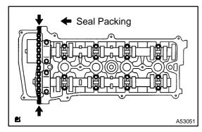
(b) Apply seal packing to 2 locations as shown in the illustration.
