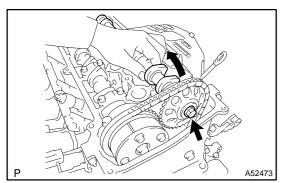
(2) Raise the No. 2 camshaft and temporarily tighten the sprocket bolt.
