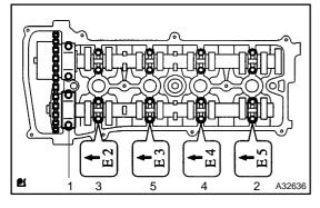
(2) Uniformly loosen and remove the No. 2 camshaft's 10 bearing cap bolts in the sequence shown in the illustration. Then remove the 5 bearing caps.
