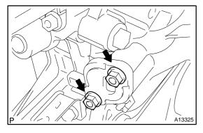
(c) Remove the 2 bolts and chain tensioner.
