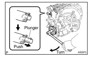
(4) Turn the crankshaft clockwise, and check that the slipper is pushed by the plunger.
