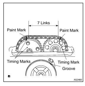
(k) Check that the timing chain paint marks are aligned with the camshaft timing sprocket timing mark and the camshaft timing gear timing mark. Also check the alignment of the pulley groove and chain cover timing mark.
