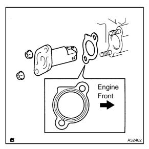
(2) Install a new gasket and the chain tensioner with the
