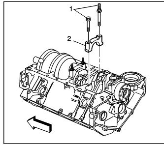
3. Install the bearings into the engine block.
