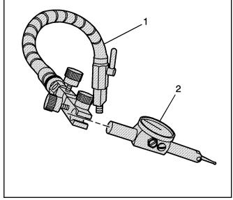
16. Insert the handle (1) to the pivot arm assembly.
