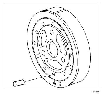
**Notice:** SIO-ID = 16580 The inertial weight section of the crankshaft balancer is assembled to the hub with a rubber type material. The correct installation procedures (with the proper tool) must be followed or movement of the inertial weight section of the hub will destroy the tuning of the crankshaft balancer.
