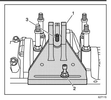
14. Align the link (1) of the pivot arm assembly on a plane (3) equal to that of the connecting rod beam (2).
