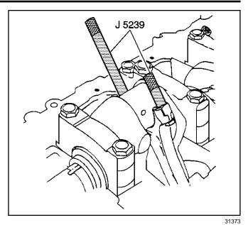
**Important:** Always assemble the connecting rod caps to the matching connecting rods.
