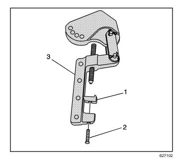
7. Install the screw (1 or 3) to the pivot arm assembly (2).
