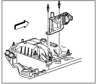
**Notice:** SIO-ID = 5005 The Linear EGR valve is an electrical component. DO NOT soak in any liquid cleaner or solvent because damage may result.
