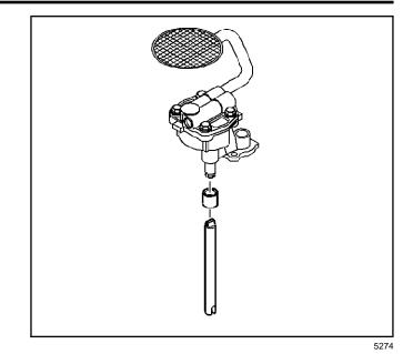
**Important:** Do not remove the oil pump screen from the pipe. The pipe and oil pump screen are serviced as a complete assembly.
