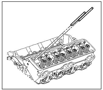
2. Remove the valve pushrods.
