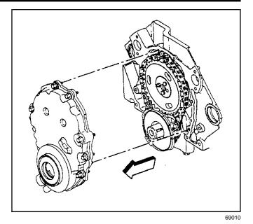
**Important:** DO NOT reuse the original crankshaft position sensor seal, O-ring. When installing the crankshaft position sensor be sure the crankshaft position sensor is fully seated and held stationary in the engine front cover crankshaft position sensor bore. A crankshaft position sensor that is not completely seated will cock in the engine front cover and may result in erratic engine operation.
