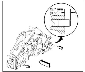
2. Remove the S type pin, and the crankshaft rear oil seal housing, if required.
