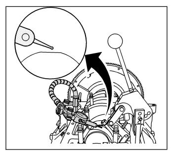
25. Rotate the fine adjustment knobs, on the dial indicator end of the swivel base, to position the tip of the indicator in contact with the connecting rod.
