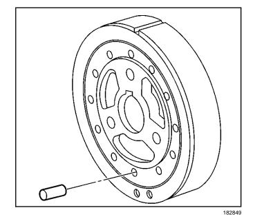
2. Remove the bolts and the crankshaft pulley.
