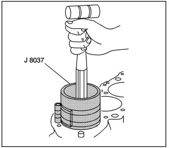
3. Install the *J* 8037 onto the piston and compress the piston rings.
