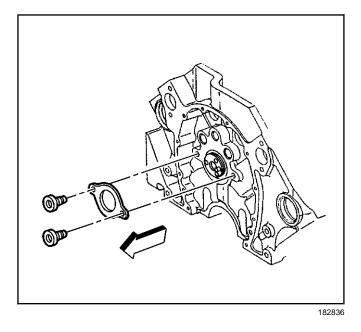
**Notice:** SIO-ID = 13833 All camshaft journals are the same diameter, so care must be used in removing or installing the camshaft to avoid damage to the camshaft bearings.
