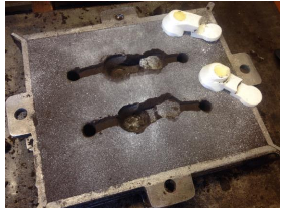
Figure 9: The 3-D printed parts and the sand casting used to pour the aluminum.
