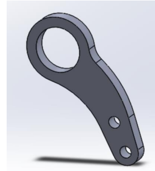
Figure 6: Final design of the front engine mounting bracket.
