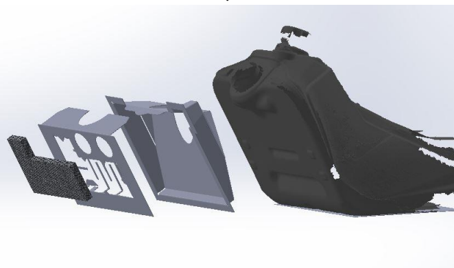
Figure 12: Fuel tank scan with initial air box, air box cover, and filter. The final design only uses the air box cavity.
