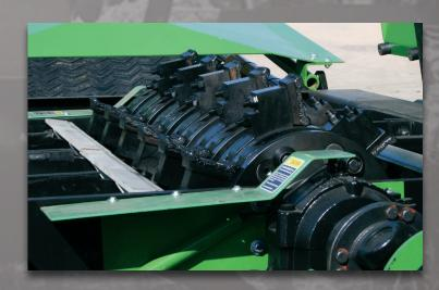
With one of the most aggressive hammermills in the industry, the ProGrind 5200 can cut through mountains of green waste at production rates of over 100 tons-per-hour. Progrind's special double-bolt hammer tips provide more durability and grinding ease, assuring high production rates, less wear on the hammermill and easy maintenance.
