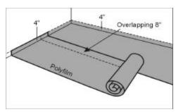
Lay out a layer of 6 mil Polyfilm and layer of foam underlayment OR 2-in-1 foam underlayment.
