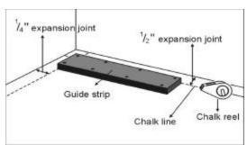
Use chalk line to trace starting line with  $\frac{1}{2}$ " expansion joint at the side and  $\frac{1}{4}$ " at row end.
