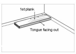
Install 1<sup>st</sup> plank along the starting line with the tongue facing out.
