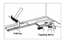
Use pull bar to tighten end joint and knocking block for the side.
