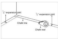
Use chalk line to trace starting line with  $\frac{1}{2}$ " expansion join at the side and  $\frac{1}{4}$ " at row ends.
