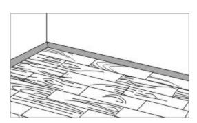
Cut plank to fit end row, allowing for ¼" expansion gap and fasten with pull bar.
