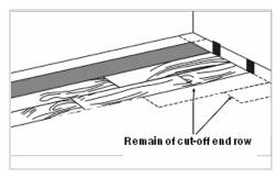
Start subsequent row using the remainder of the cut-off plank from previous row.
