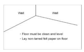
Lay 15 lb non-tarred felt paper or equivalent (with 3" to 4" overlapping end) in the direction of the boards using staples. This will reduce the normal mechanical friction between materials and facilitate installation.
