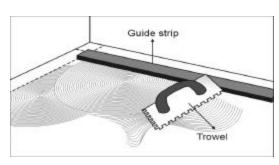
Use the trowel and apply adhesive at a 45° angle from the starting line outward. Install the first plank along the guide strip with tongue facing you and the groove facing the starting wall.
