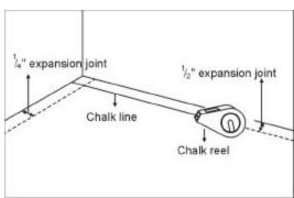
Use chalk line to trace starting line with  $\frac{1}{2}$ " expansion joint at the side and  $\frac{1}{4}$ " at row end.
