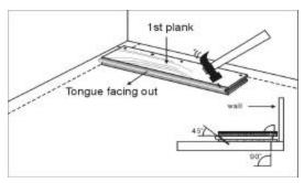
Install the 1<sup>st</sup> plank along the starting line with the tongue facing out and grove facing the wall.
