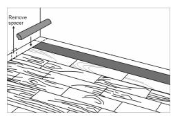
Once the entire surface is covered, remove the expansion spacers to install molding to cover the expansion joint.
