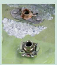
AIRCRAFT CARGO SIDE PANEL (Top: Riveted nut plate / Bottom: ForceTec)
