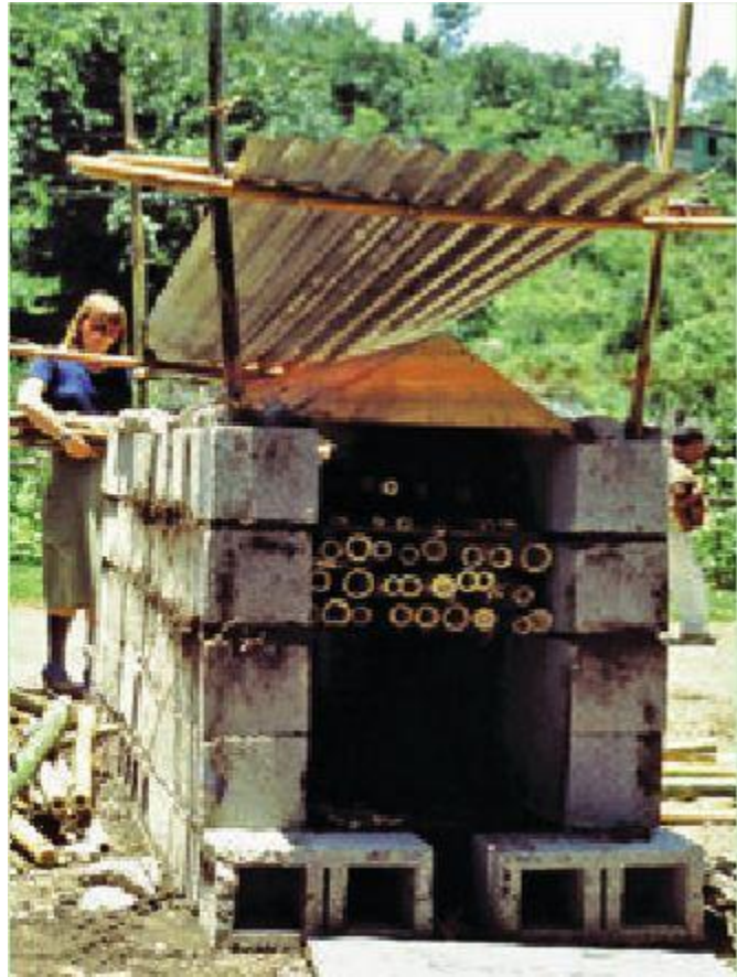
Figure 74. High Temperature Drying with Wood Fire, from (Minke 2012)
