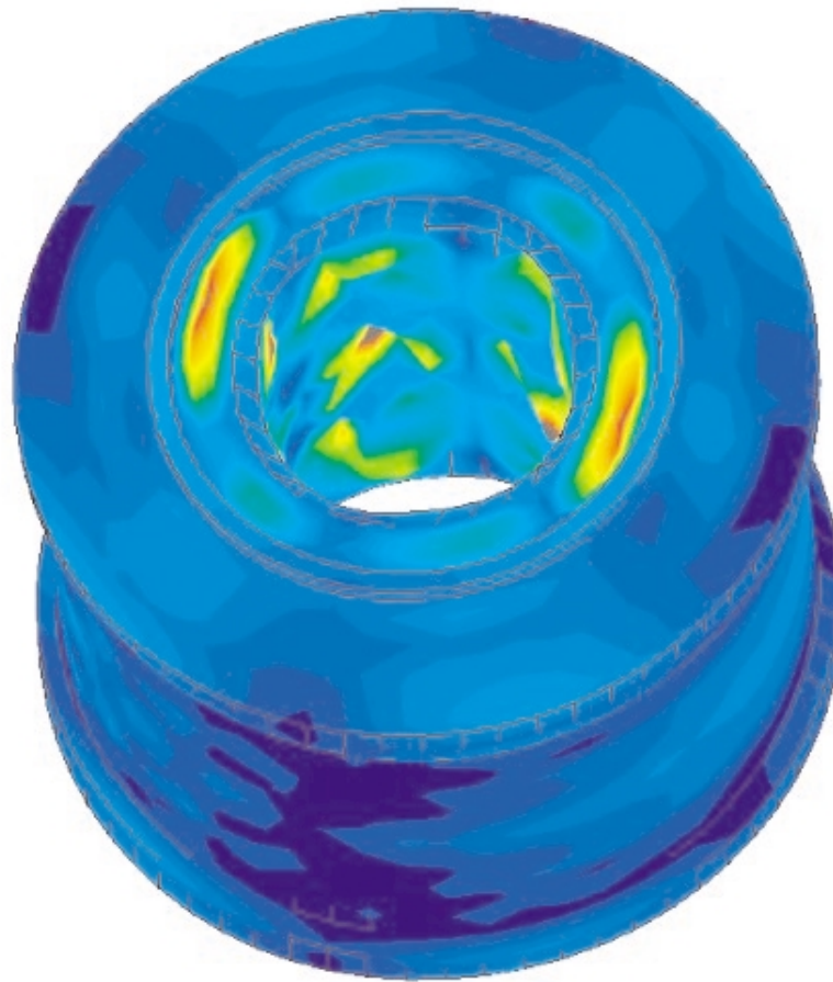
Figure 1 Displacement contours of the magnet.
