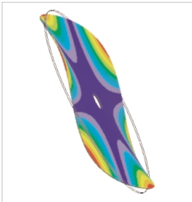
Figure 1 One of the higher eigenmodes of the hot saw.
