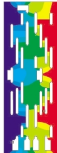
Figure 2 Calculation of local distortions (max. 10 nm) of a 6x17 \mu\text{m} mask area under applied stress. The effective stiffness is calculated by averaging over the area.
