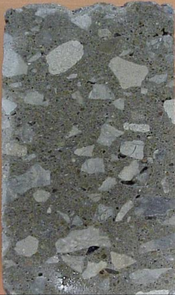
Iowa DOT C-5WR Mix (Gap Graded)
