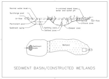
Sediment trap/constructed wetland
