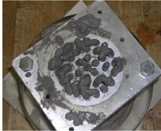
Figure 3.15. Detail of modified base plate: (a) pattern of 0.25” holes; (b) example of shale specimen after extrusion.
