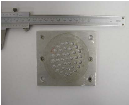
Figure 3.15. Detail of modified base plate: (a) pattern of 0.25” holes; (b) example of shale specimen after extrusion.
