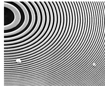
Zone plate x-ray "lens" Outer ring spacing \sim 35 nm
