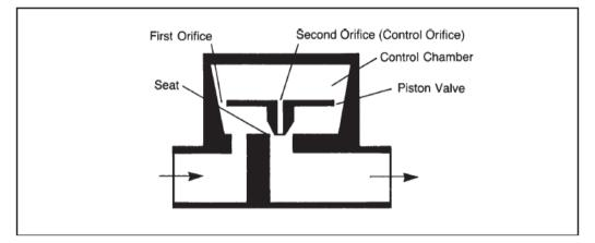
VARIABLE-ORIFICE (PISTON) TRAP (COURTESY OF YARWAY CORPORATION) Fig. 2
