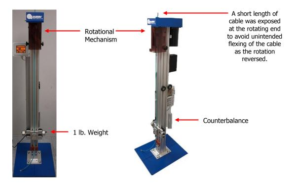
Next the cord was clamped in the test fixture using care not to crush the cable.
