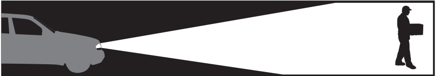
High beam headlights can reveal objects up to a distance of at least 450 feet and are most effective for speeds faster than 25 mph.
