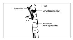
Reroute the pipings and the drain hose across the back of the chassis.
