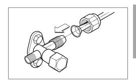
Finally, tighten the flare nut with torque wrench until the wrench clicks.
