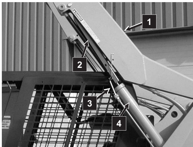
Fig. 5-14: Lift Arm Raised and Support Device Engaged
