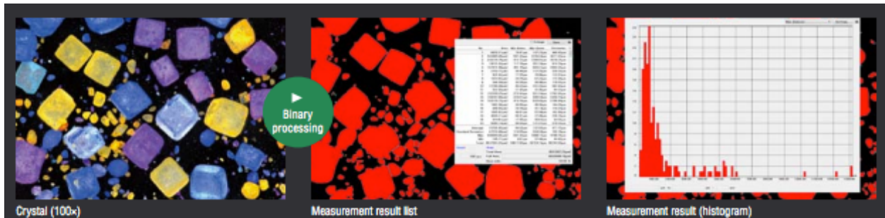
Figure 2: Automatic area measurement feature of Keyence microscope.
