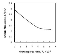
Figure 6. Anchor force ratio,  $R_F$  due to various values of grouting area ratio,  $R_g$ .
