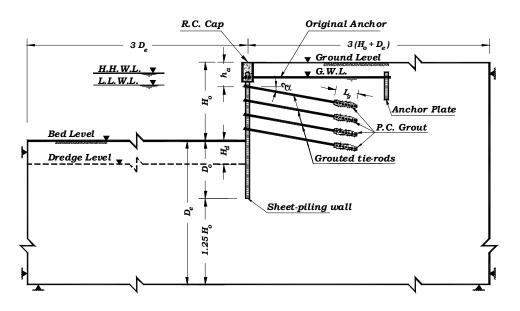
Figure 1. Geometry of Multi-Anchored-Sheet Pile System.
