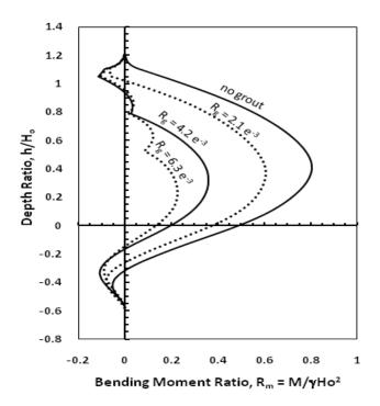
**Figure 3.** Bending moment ratios,  $R_m$  along sheet-piling quay wall due to various values of grouting area ratio,  $R_a$ .
