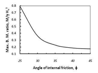
**Figure 7.** Maximum bending moment ratio,  $R_m$  versus backfill soil angle of internal friction,  $\phi$ .
