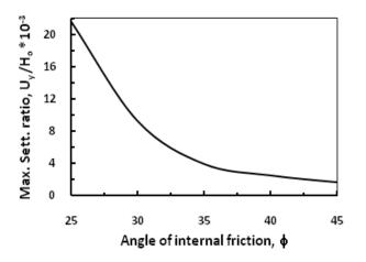
**Figure 9.** Maximum settlement ratio,  $R_{uy}$  versus backfill soil angle of internal friction,  $\phi$ .
