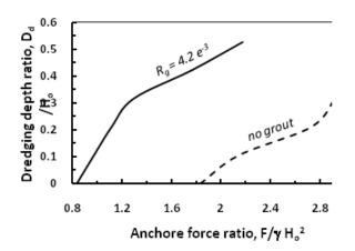
Figure 12. Maximum anchor force ratio,  $R_F$  versus dredging depth ratio,  $R_d$ .
