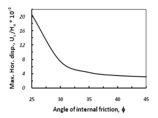
**Figure 8.** Maximum horizontal displacement ratio,  $R_{ux}$  versus backfill soil angle of internal friction,  $\phi$ .
