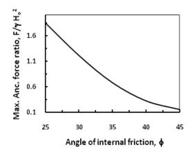
Figure 10. Maximum anchor force ratio,  $R_F$  versus backfill soil angle of internal friction,  $\phi$ .
