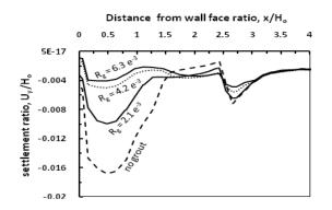
Figure 5. Ground surface settlement ratio,  $R_{uy}$  along sheet-piling quay wall due to various values of grouting area ratio,  $R_{g}$ .
