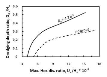
Figure 13. Maximum horizontal displacement ratio,  $R_{\text{ux}}$  versus dredging depth ratio,  $R_{\text{d}}.$
