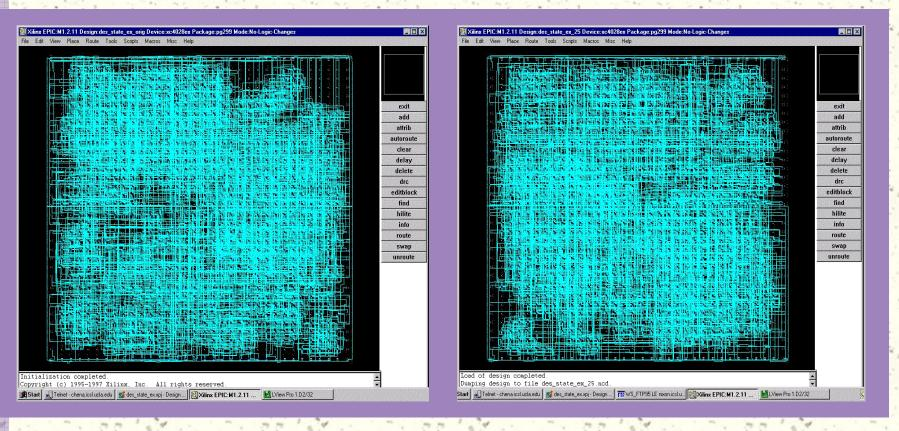
DES: Same functionality, area, and performance with a 4768-bit watermark embedded in the FPGA design
