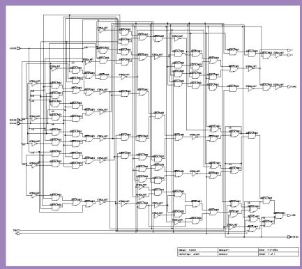
A 4-bit ALU: Original gate-lever circuit and the same design with message "UMCP TERPS" embedded.
