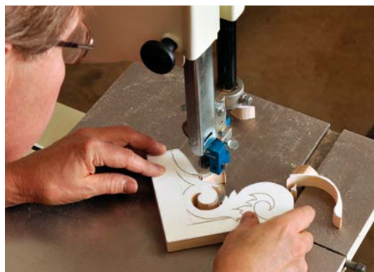
Equipped with a narrow blade, a bandsaw can cut accurate circles and tight scroll patterns with precisely square edges.
