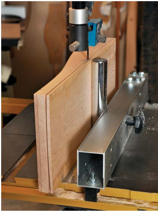
The single-point bar attached to this rip fence allows resawing of crooked or curved pieces.
