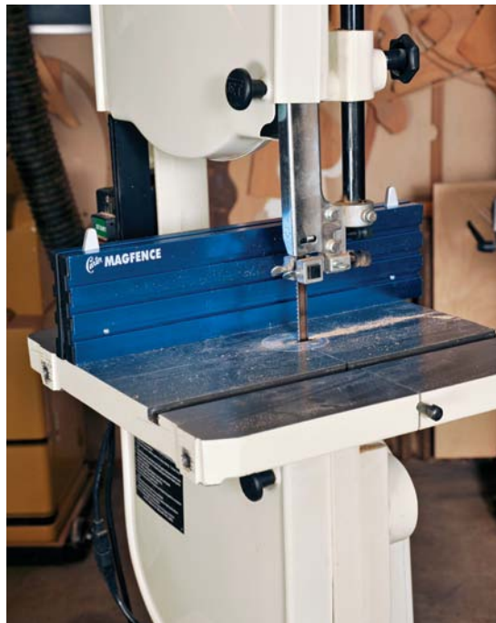
Rare earth magnets allow easy positioning of Carter’s Magfence™ without the need for clamps or a fence rail.
