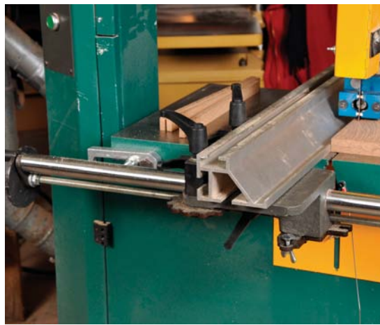
This aftermarket fence from Laguna® Tools can be quickly adjusted to accommodate blade drift. It also includes a feed screw for accurate incremental fence positioning.
