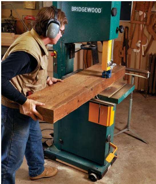
A bandsaw can easily rip thick timbers, even on a 120-volt circuit.
