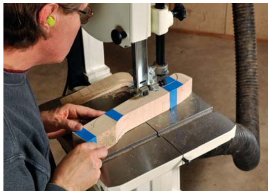
Sawing complex shapes and compound curves in thick wood is one of the bandsaw's unique abilities.
