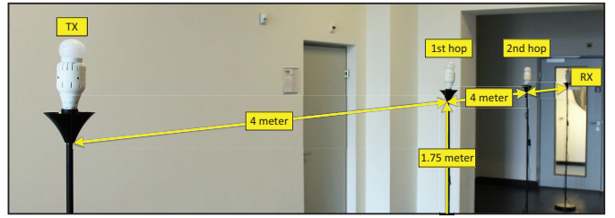
Fig. 6. Testbed setup. The light bulbs are placed in floor lamps 1.75 meter above floor level and line up each 4 meters apart.
