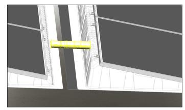
Take the two engaged Wire Duct components and connect them together by placing one unit inside the other in a telescoping fashion. Adjust the completed Wire Duct assembly to the appropriate length according to the inter-row spacing for the array.
