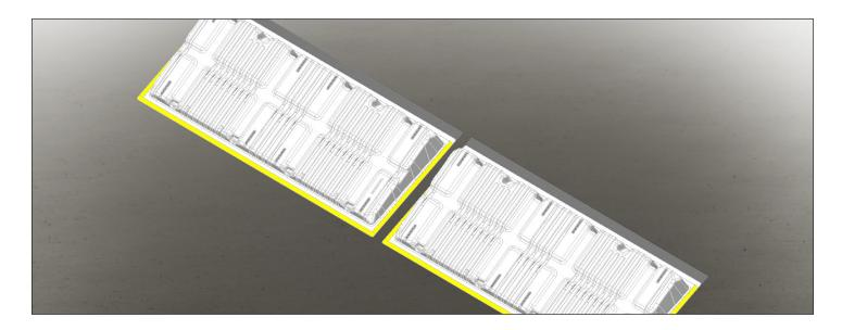
ENRGY Curbs in the field or north row of an array may overlap the neighboring south curb's TPO membrane depending on the inter-row spacing. Ensure the top surface of the ENRGY Curb's TPO membrane is properly cleaned before the peel-and-stick tape is overlapped. Tape application should be performed in temperatures above 50°F (10°C) to ensure best results.
