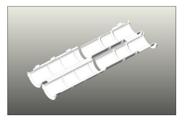
Take each wire duct component and fold along the hinge or connected edge. Fold until each locking mechanism snaps and engages into place. The locking mechanisms are meant for single use and should not be disconnected once engaged.
