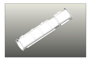
There are two mating slots on every ENRGY Curb 10-01 and four mating slots on every ENRGY Curb 10-02 that can be utilized. Place the Wire Duct assembly into the mating slots on the south and north edges of the ENRGY Curbs where inter-row wiring is required. Wire Ducts may not be required at all mating slots; please refer to the approved design documents for your wiring layout.
