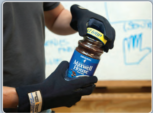
Kraft Foods used GTRI's arthritis simulation gloves to verify that the Maxwell House instant coffee EZ Grip lid was accessible by consumers who have difficulty opening jars with regular caps.
