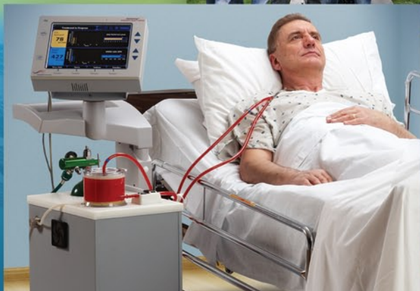
ALung is commercializing artificial lung devices that can replace ventilators in patients with acute respiratory failure
