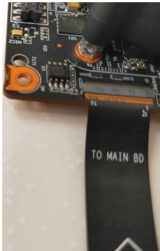
Figure 3-13 Inserting the fastener
