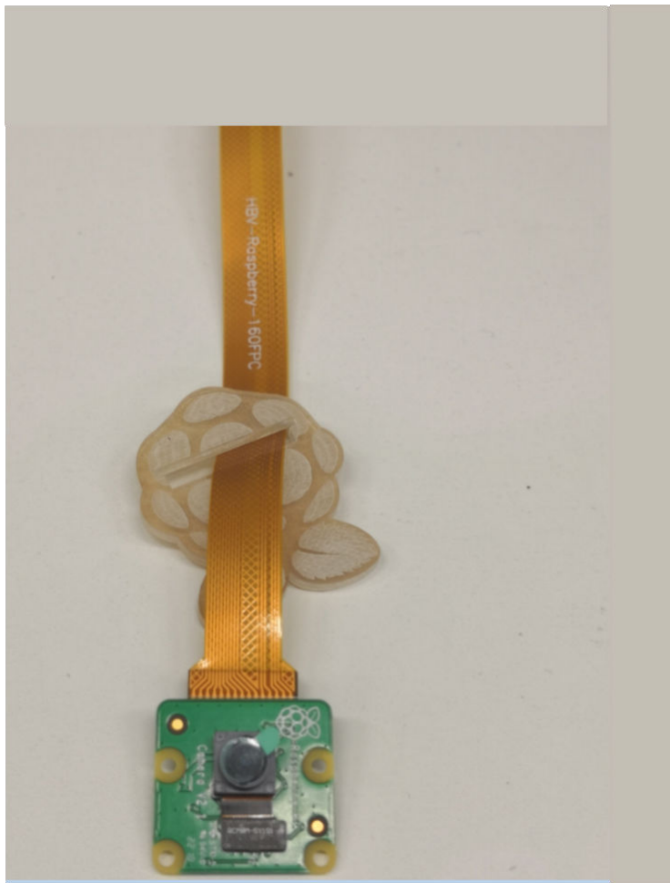
Figure 3-6 Installing the fixing film
