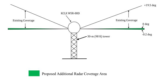
Figure 4: Drawing Showing Proposed Additional Radar Coverage
