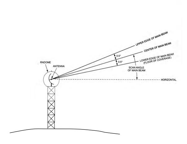
Figure 3: Schematic of WSR-88D Main Beam
